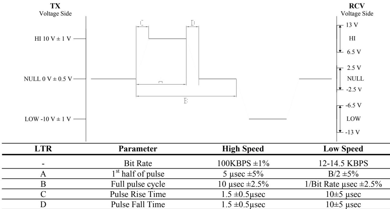
**Figure 2: ARINC 429 Waveform Characteristic (top) and ARINC 429 Output Signal Tolerances (bottom)**
