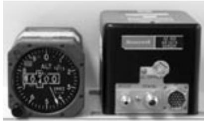
*Honeywell Air Data and altimeter removed from a CitationJet to install RVSM equipment.*
