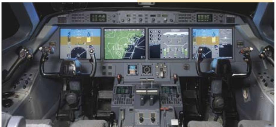
*Built on Honeywell’s Primus Epic avionics suite, Gulfstream’s PlaneView Cockpit offers new features and functions, such as enhanced vision.*
