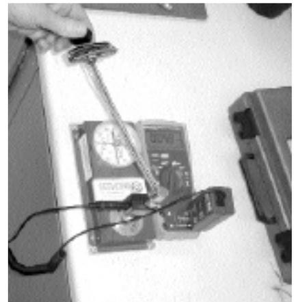
*Measuring the calibration of a torque wrench using two standards*
