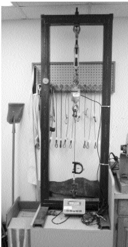
*Device used for tension meter calibrations*
