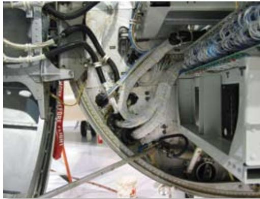
*Premier Air Center/ West Star Aviation gives this Falcon 50 the four-tube EFI-890R installation, including Vision-1, Class A TAWS, dual UNS-1E FMS, P-880 radar, Collins AH-3000 AHRS, dual Universal radio control units, and dual Baker M-1035 audio panels.*
