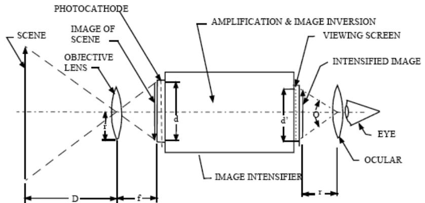
**Figure C-1. Diagram of an image intensifier.**
