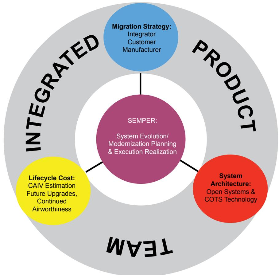
The SEMPER model has evolved from a series of systems upgrade planning activities conducted in support of commercial, civil and government aircraft. The SEMPER model embraces both systems engineering and business planning processes and focuses on structuring relevant information for the customer to use during the modifica-
