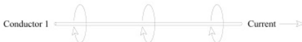
**Figure 4** Magnetic field created by current flow.
