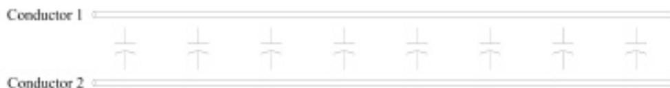
**Figure 2** Two parallel wires acting as plates of a capacitor.
