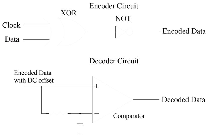
**Figure 4 ARINC-708 Wx Bus Manchester Encoding/Decoding**
