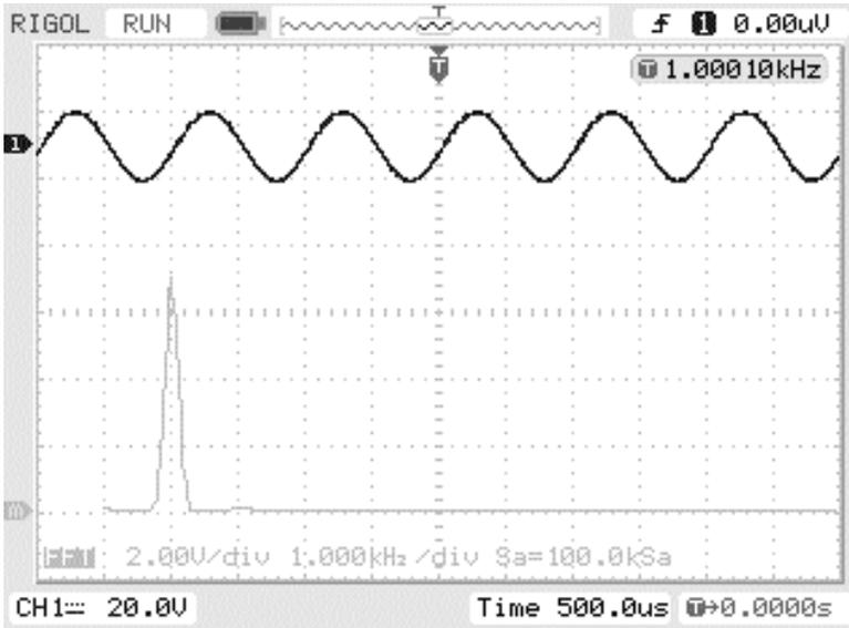
**Figure 2: Sine Wave Time and Frequency Domain**
