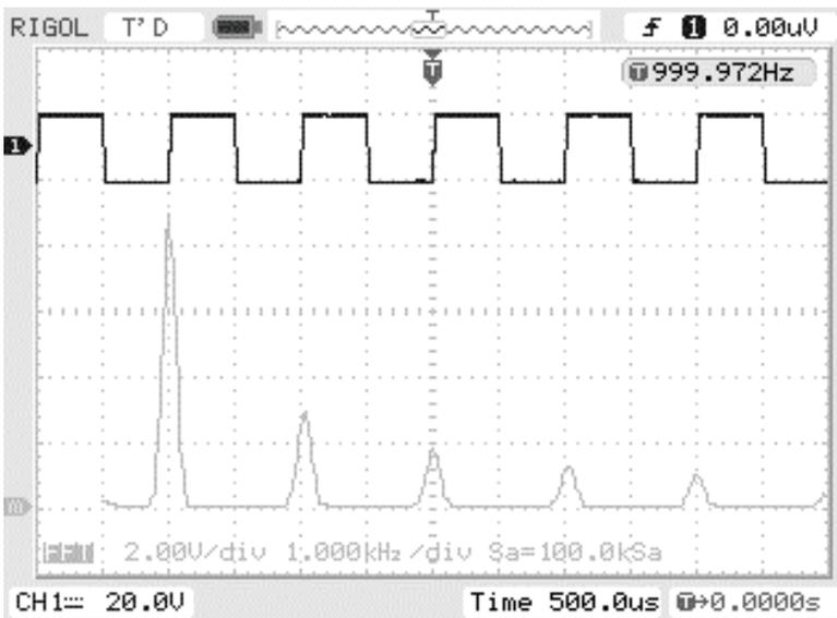
**Figure 3: Square Wave Time and Frequency Domain**
